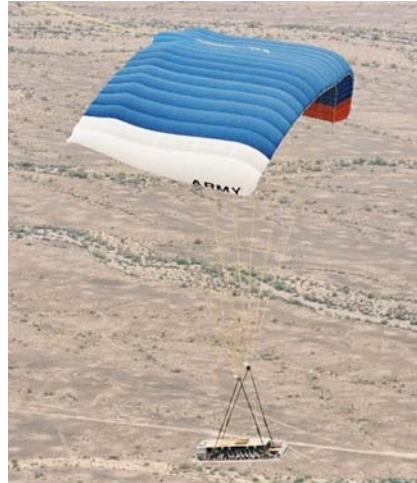
Figure 18: 10,000-pound Payload Delivered by a 4200-foot 2 Parafoil.
